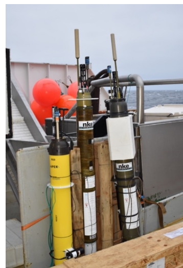
Cruise track and location of Argo float deployments (left figure) and three float types from left to right (right figure, photo: Tor de Lange): bio, deep, and BGC floats.
